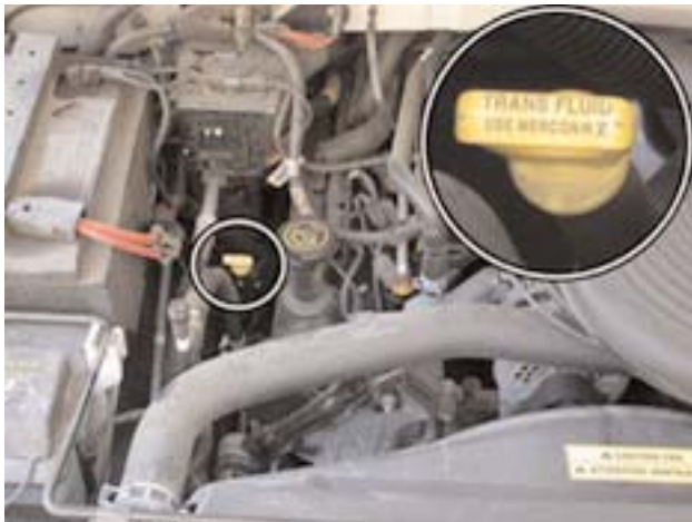
Transmission dipstick on a RWD.
